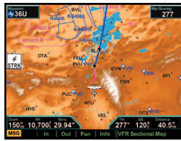
Custom map feature allows the pilot to overlay some or all of the MX20 features.
