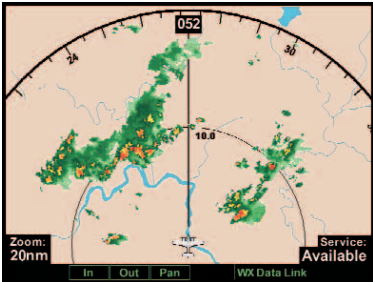
FIS map displays graphical NEXRAD weather along the route and nationwide weather summary charts.
