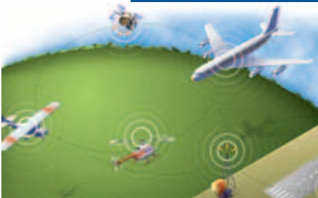
Airborne ADS-B broadcasts aircraft position, altitude, vector and other information for enhanced air traffic management.
