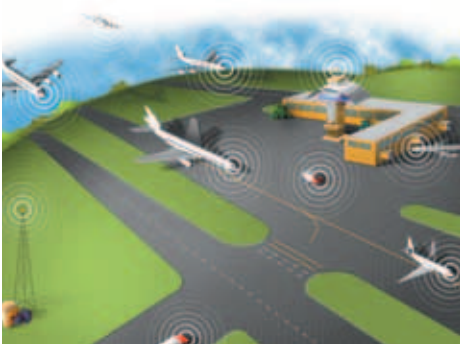
In the future, ADS-B will enable better monitoring of surface traffic on airport taxiways and runways.
