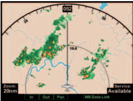
Using the ADS-B datalink, pilots can view graphical NEXRAD weather and nationwide weather summary charts uplinked from the ground to their cockpit display.
