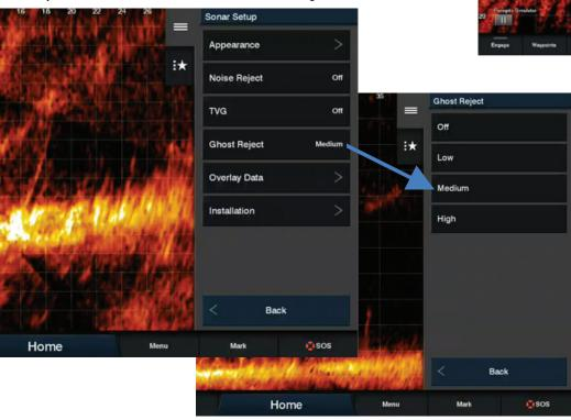
The new "Ghost Reject" setting steers more of the transmit power forward, which reduces the bottom return strength and therefore the interference that generates the interference that creates the Ghost Tree.
