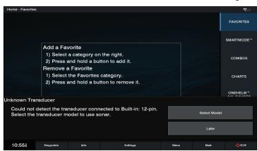
If the user performs a software update on a chartplotter connected to one of the affected transducers, they will be prompted to manually select the transducer following the update. The transducer models most likely to match the connected transducer are shown at the top of the selection list.
