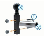
2 Tighten the nuts to secure the base.
