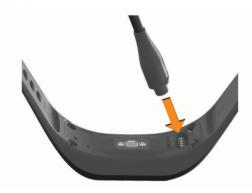
**3** Plug the USB cable into a power source to turn on the device (*Charging the Device*, page 8).
