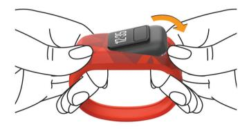
2 Insert the device into the flexible silicone band by stretching the band material around the device. The arrow on the device must be aligned with the arrow inside the band.
