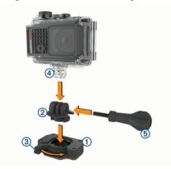
3 Allow the base to bond to the mounting surface for at least 24 hours.
