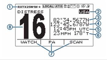
Radio system status, settings, and alerts International, Canadian, or USA frequency band Latitude<sup>1</sup> Longitude 1 Time<sup>1</sup> Speed over ground (SOG) or course over ground (COG) <sup>2</sup> Soft-key functions change depending on your current activity 8 Working channel
