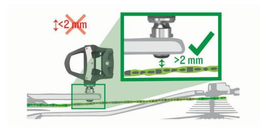
**NOTE:** Garmin recommends 2 mm or more between the pedal and the chain. If the pedal rubs the chain, you can add one washer (included) between the spindle and the crank arm to increase clearance. To maintain an equal q factor, you can add one washer to the left pedal spindle. Do not use more than one washer on each pedal.
