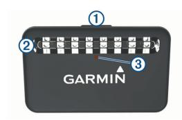
The taillight LEDs ② fill horizontally to indicate the battery level. The status LED ③ indicates additional device information.
