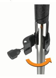
**4** Tighten the thumbscrew so the device does not move during use.
