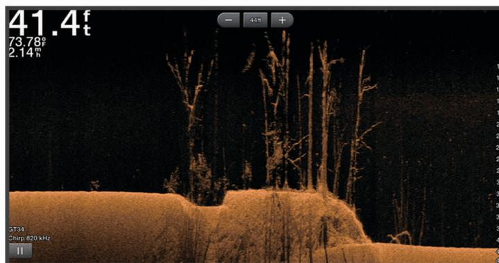
Traditional transducers emit a conical beam. The Garmin ClearVü scanning sonar technology emits a beam similar to the shape of the beam in a copy machine. This beam provides a clearer, picture-like image of what is beneath the boat.
