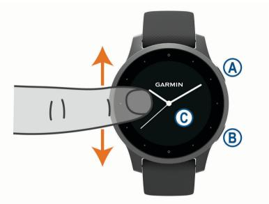
Action button: Press to turn on the device.
