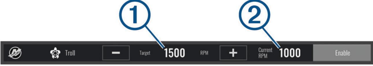
The screenshot shows a control panel for the Mercury Troll function. It includes a minus sign button, a 'Target' display showing '1500 RPM', a plus sign button, a 'Current RPM' display showing '1000', and an 'Enable' button. Two callout boxes with numbers 1 and 2 point to the minus sign and the 'Current RPM' display respectively.
