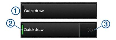
A green light on an option indicates the option is enabled 2.
