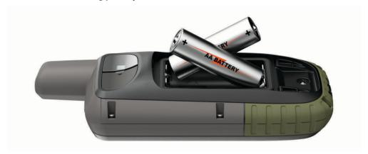
3 Replace the battery cover, and turn the D-ring clockwise.
