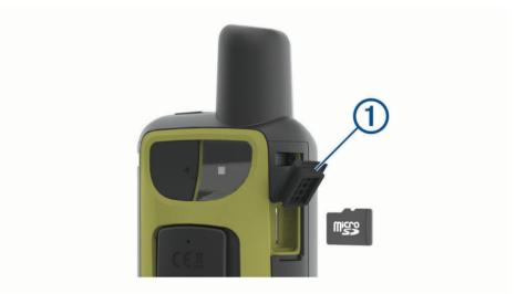
2 Insert the memory card with the gold contacts facing the front of the device.
