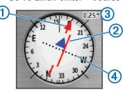
The course pointer ① indicates your relationship to the course line leading to the destination. The course deviation indicator (CDI) ② provides the indication of drift (right or left) from the course. The scale ③ refers to the distance between dots ④ on the course deviation indicator, which tell you how far off course you are.
