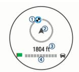
The destination indicator ① shows the direction of your destination relative to the direction you are moving ②. When the destination indicator appears at the top of the circle, you are heading toward your destination. The remaining distance to your destination ③ appears below the circle. The progress bar ④ shows your progress toward your destination.
