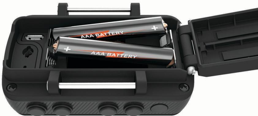
**NOTE:** You should verify the gasket and battery compartment are free of debris.
