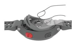
There should be no gaps between the light seal and the back of the device.
