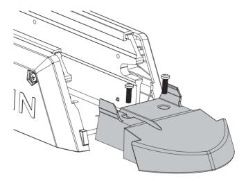
4 Install a replacement mount bumper, and secure it to the mount base using the screws provided with the replacement part.
