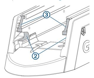
8 Apply a synthetic or marine grade, general-purpose grease to the upper surface ③ of the latch receivers on the front of the mount base, so the locking mechanisms slide smoothly into the receivers.
