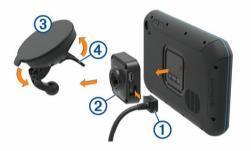
2 Press the mount (2) onto the suction cup (3) until it snaps into place.
