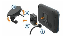
2 Press the mount ② onto the suction cup ③ until it snaps into place.
