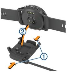
4 With the contacts aligned, place the device into the cradle 2 and release the arms to hold the device in place.
