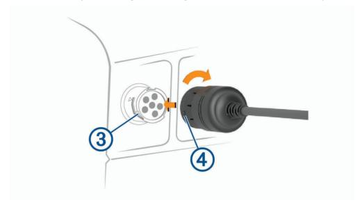
5 Turn the lock ring clockwise until it locks into the vehicle port.
