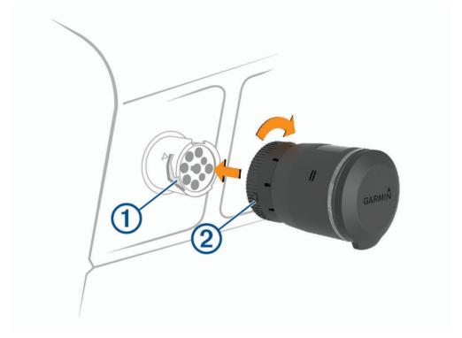
3 Turn the lock ring clockwise until it locks into the diagnostic port.
