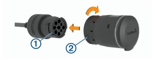
3 Turn the device lock ring clockwise until it locks into the adapter cable.
