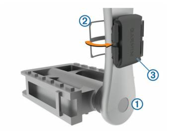
4 Rotate the crank arm to check for clearance.
