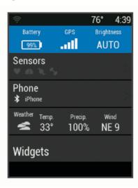
The status page appears. A flashing icon means the device is searching for a signal. A solid icon means the signal was found or the sensor is connected.
