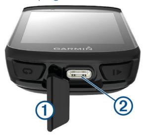
2 Plug the small end of the cable into the charging port on the device.
