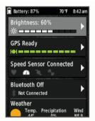
The status page appears. A solid icon means the signal was found or the sensor is connected.
