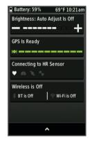
The connections screen appears. A flashing icon means the device is searching. You can select any icon to change the settings.
