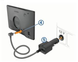
4 Plug the other end of the vehicle power cable (5) into a power outlet in your vehicle.
