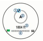
The destination indicator ① shows the direction of your destination relative to the direction you are moving ②. When the destination indicator appears at the top of the circle, you are heading towards your destination. The remaining distance to your destination ③ appears below the circle. The progress bar ④ shows your progress towards your destination.
