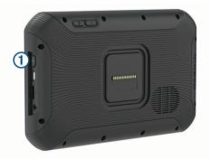
To put the device in power saving mode, press the power key while the device is on.
