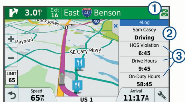
Diagnostic and malfunction indicator. Select to view detailed ① information about diagnostic or malfunction alerts (*Viewing .(17 Diagnostics and Malfunctions*, page
