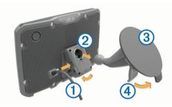
2 Press the mount ② onto the suction cup ③ until it snaps into
