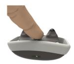
The base unit begins searching for the dog collar device. When paired, a preset boundary of 15 m (50 ft.) displays on the base unit.
