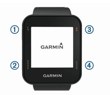
UP O Hold to turn the device on and off. Select to scroll through menus and settings. During play, select to scroll through hazards, layups, and doglegs.
