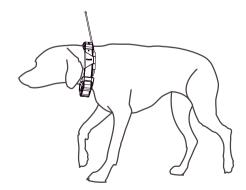
3 Wiggle the device to work the contact points through the dog's coat. **NOTE:** The contact points must have contact with the dog's skin to be effective.
