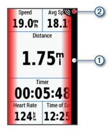
The vehicle position LED ① moves up the column as a vehicle gets closer to your bike. The threat level LED ② changes color based on the potential level of threat. Green indicates no vehicle is detected. Amber indicates a vehicle is approaching. Red indicates a vehicle is advancing at a high rate of speed.
