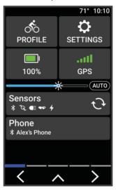
The status widget appears. A flashing icon means the device is searching. A solid icon means the signal was found or the sensor is connected.
