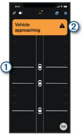
The vehicle position ① moves up the screen as a vehicle gets closer to your bike. The threat level banner ② changes color based on the potential level of threat. Green indicates no vehicle is detected. Amber indicates a vehicle is approaching. Red indicates a vehicle is advancing at a high rate of speed.
