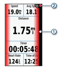
The vehicle position LED ① moves up the column as a vehicle gets closer to your bike. The threat level LED ② changes color based on the potential level of threat. Green indicates no vehicle is detected. Amber indicates a vehicle is approaching. Red indicates a vehicle is advancing at a high rate of speed.
