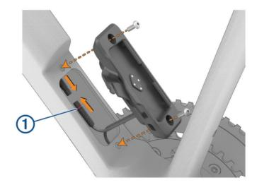
**NOTE:** Avoid touching or moving the O-ring ① to ensure the cables connect and seal correctly.
