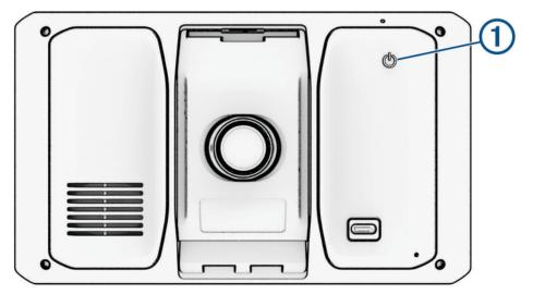
• To put the device in power saving mode, press the power button while the device is on. While in power saving mode, the screen is off and the device uses very little power, but it can wake instantly for use.
