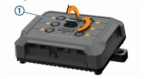
2 Pull the front cover off of the device.
