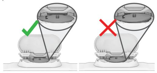
10 Check the battery cover alignment to ensure it is fully closed and locked into place.
