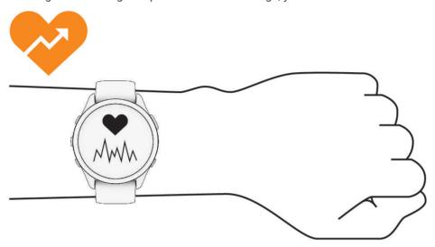
**NOTE:** The optical sensor is located on the back of the watch.
