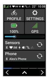
The status widget appears. A flashing icon means the device is searching for a signal. A solid icon means the signal was found or the sensor is connected. You can select any icon to change the settings.
