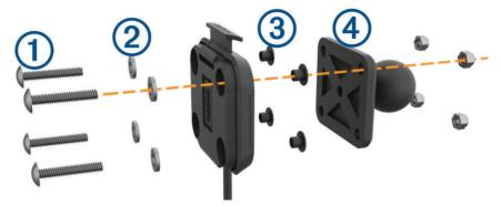
2 Tighten the nuts to secure the base plate.
