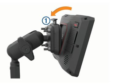
2 Push the top of the device forward until it snaps into place.
