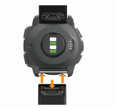
**NOTE:** Make sure the band is secure. The latch should close over the watch pin.
