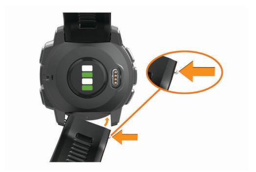
NOTE: Make sure the band is secure. The watch pin should align with the holes on the device.
