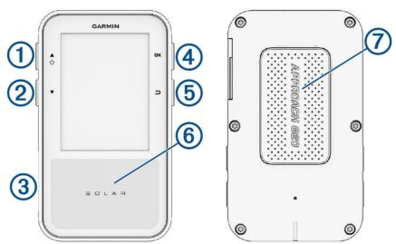
1) A (): Hold to turn the device on and off.
