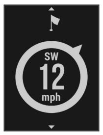
The arrow points to the wind direction relative to the pin.
