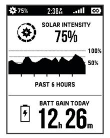
The device goes into a low power, battery charging mode, and a screen with solar charging statistics appears. The display turns off automatically when sunlight is no longer detected.
