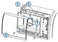
**6** Place the bezel ® on the front of the dock. Magnets hold the bezel in place.
