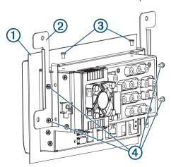
3 Using the included screws, secure each bracket to the top 3 and the sides 4 of the dock.
